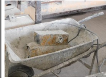
#41: Vibrating Needle with Converter
