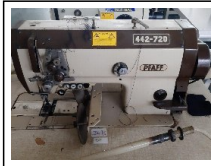
#30: Machine 2 Pfaff Disengageable Needles 12 mm
